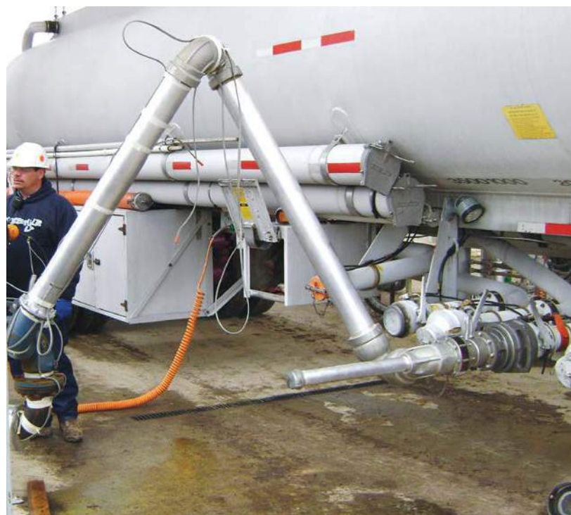
"A"-frame-style arm is designed for bottom-loading tank trucks. /
