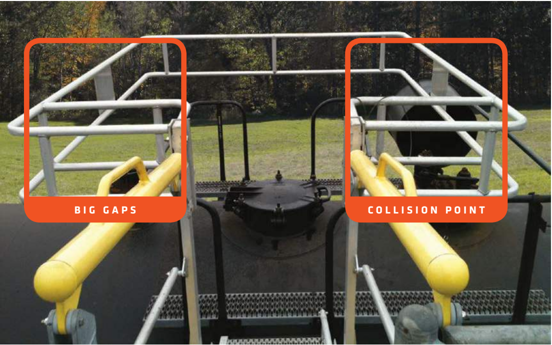
OFFSET CRASH BOX APPLICATION / Standard-width gangways and cage do not function well in this type of application. /
