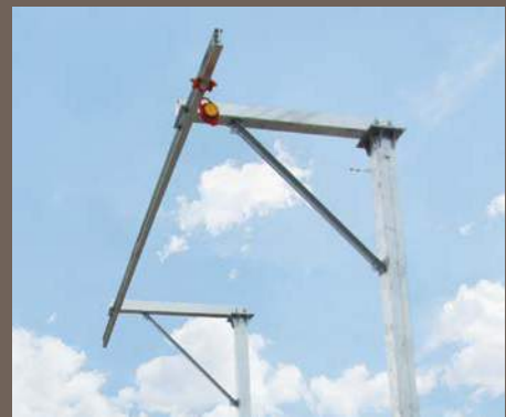
Trolley beam fall protection system for accessing trucks or railcars. /
