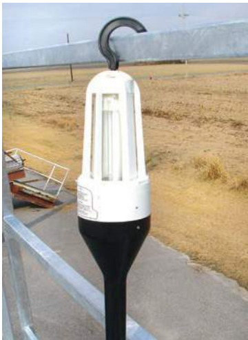
Class one inspection light for checking trucks & railcars.
