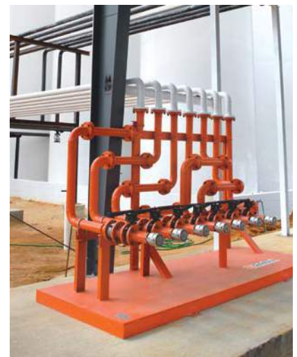
Truck unloading skid for incoming feedstock, fuel & chemicals. /
