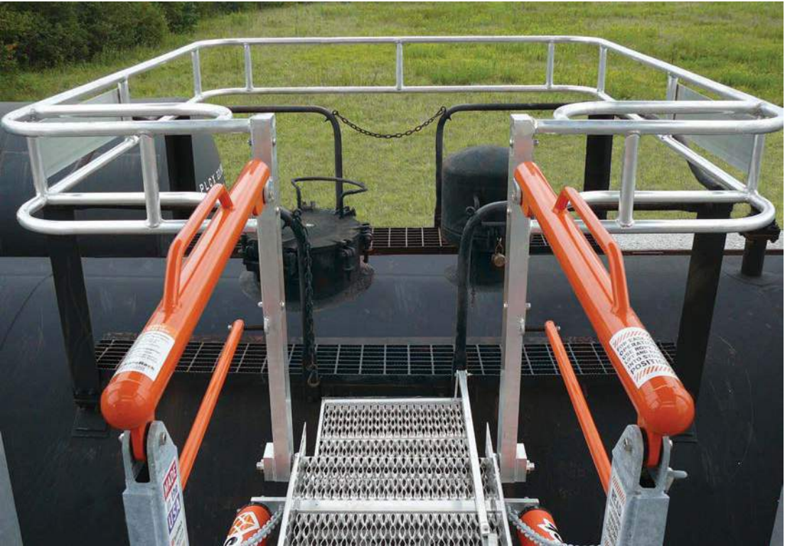
SYMMETRICAL CRASH BOX APPLICATIONS / Standard-width gangways function well with this tank car. /
