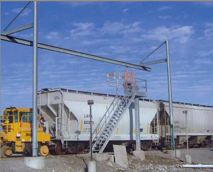
Trolley beam system integrated with SafeRack access platform. /
