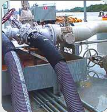
Hose in service; note the gradual bend achieved off of the horizontal connections
