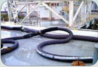
Hose in service; note the gradual bend achieved off of the horizontal connections
