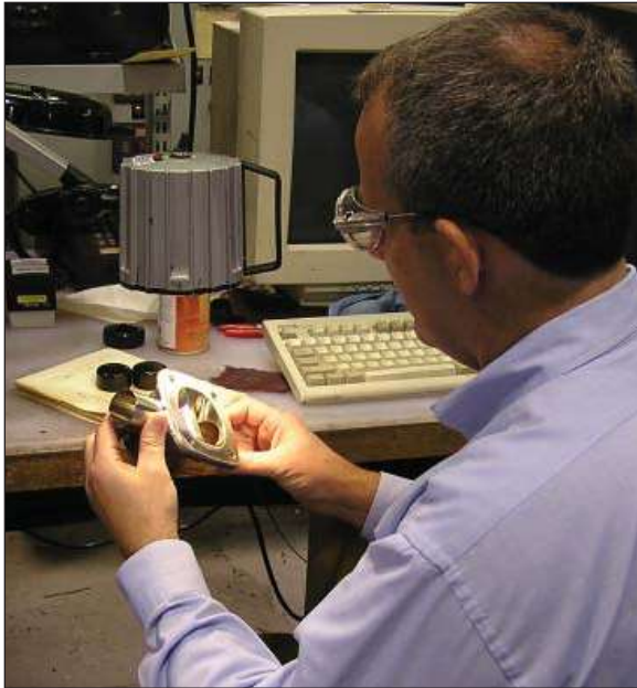
Profilometer Check for Valve Surface Finish
