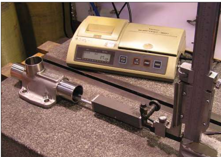
Profilometer Check for Valve Surface Finish
