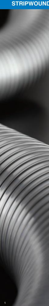
Stripwound metal hose is a rugged product made from a strip of steel that is profiled and continuously wound around a mandrel to form a hose. Hose Master's proprietary manufacturing process yields an extremely consistent and balanced profile that maximizes strength and flexibility. Stripwound hose is used as a guard, exhaust hose, and for the transfer of dry bulk materials.
