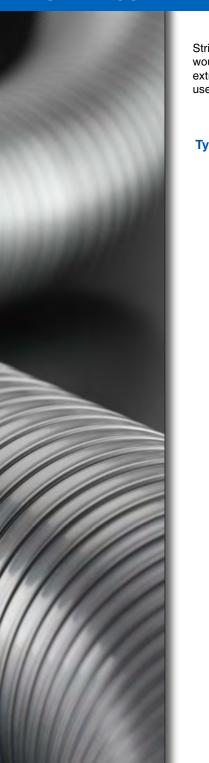
Stripwound metal hose is a rugged product made from a strip of steel that is profiled and continuously wound around a mandrel to form a hose. Hose Master's proprietary manufacturing process yields an extremely consistent and balanced profile that maximizes strength and flexibility. Stripwound hose is used as a guard, exhaust hose, and for the transfer of dry bulk materials.
