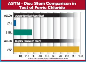
Sure Seal's standard is a 255 duplex stainless which is more corrosion resistant and almost twice as strong as all other butterfly valve manufacturers standard 316 stainless steel. This eliminates shaft twisting and water hammer damage which other butterfly valve manufacturers have to make their disc thicker to handle water hammer which also reduces the CV of their valve. With Sure Seal's standard no
