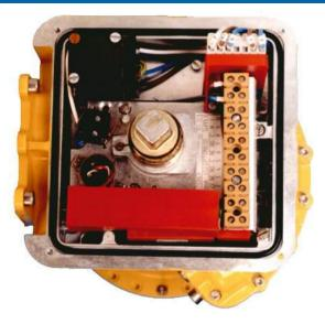
An electronic circuit and a feedback potentiometer are fitted inside the standard actuator control box. The circuit is a high stability linear comparator, which switches the actuator pump and solenoid valves via solid state mains switches in response to the difference between the actual position measured by the potentiometer and the intended position given by the 4-20mA signal. Limit switches prevent the actuator driving against its own endstop, whatever the signal may be.
